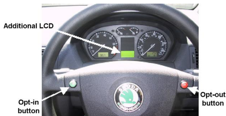
Figure 12 – The ISA HMI developed in the UK ISA project. Image source: Lai and Carsten (2012)
