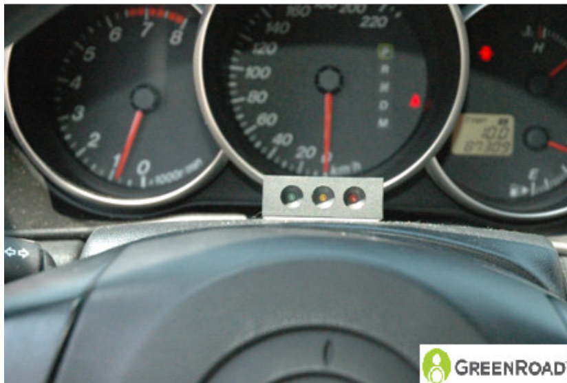
Figure 10: IVDR real-time feedback unit
